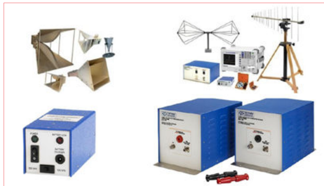
Figure 7: examples of radiated and conducted emission measurement equipment
